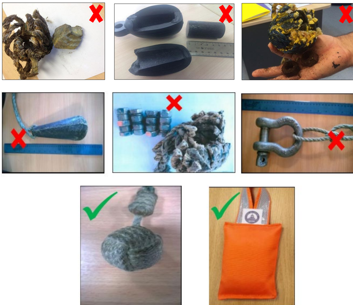
Figure 7. Examples of good and bad seamanship practices of heaving lines.
